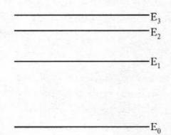
Electron transitions occur between all of these levels to produce emission lines in the spectrum of this atom.
